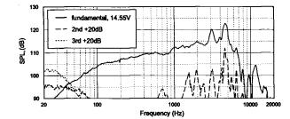
*Figure 3.* 2020H at one-tenth rated power (30 W); 2nd (dashed) and 3rd (dotted) harmonics raised 20 dB.
